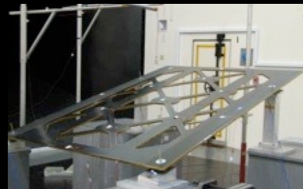
Lattice Configuration Acoustic Test Panel to validate Unitized Pallet Structure loads
