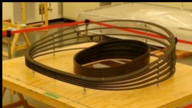
Core Model for Rim deployment and inner membrane surface development (Hub & Rim shown)
