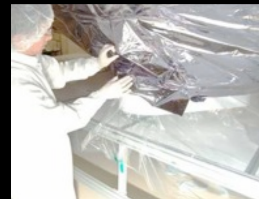
EPF-2 Membrane revealed core shape issues
