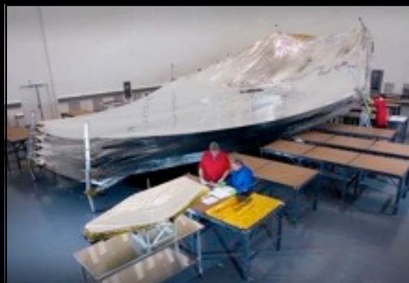
EPF-0 provided first evaluations of full scale membrane
