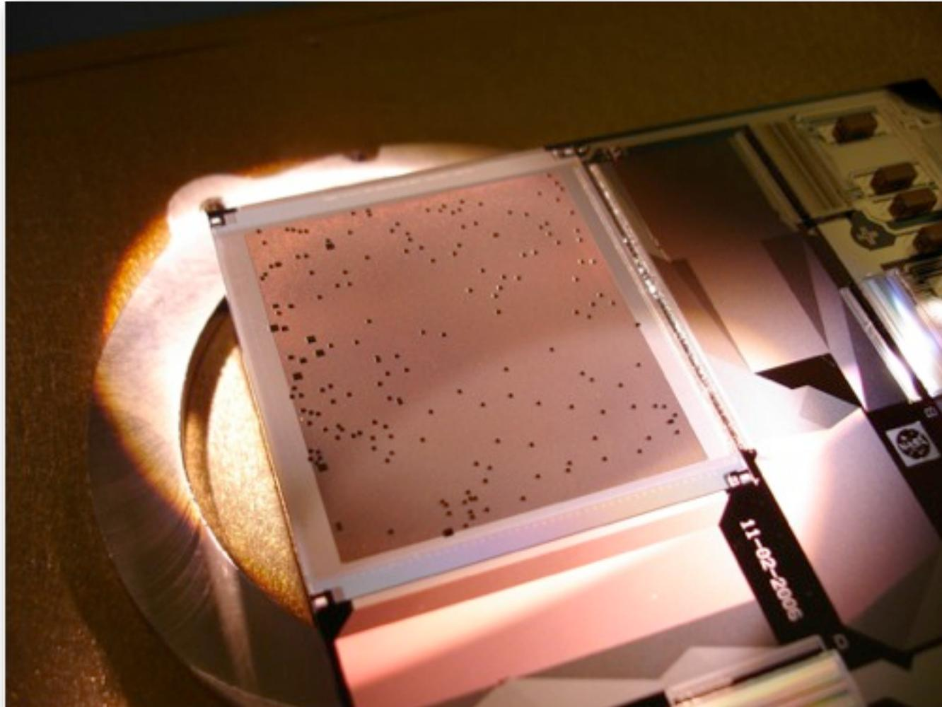
Trade each failed open shutter for 3x3 patch of failed closed ones
