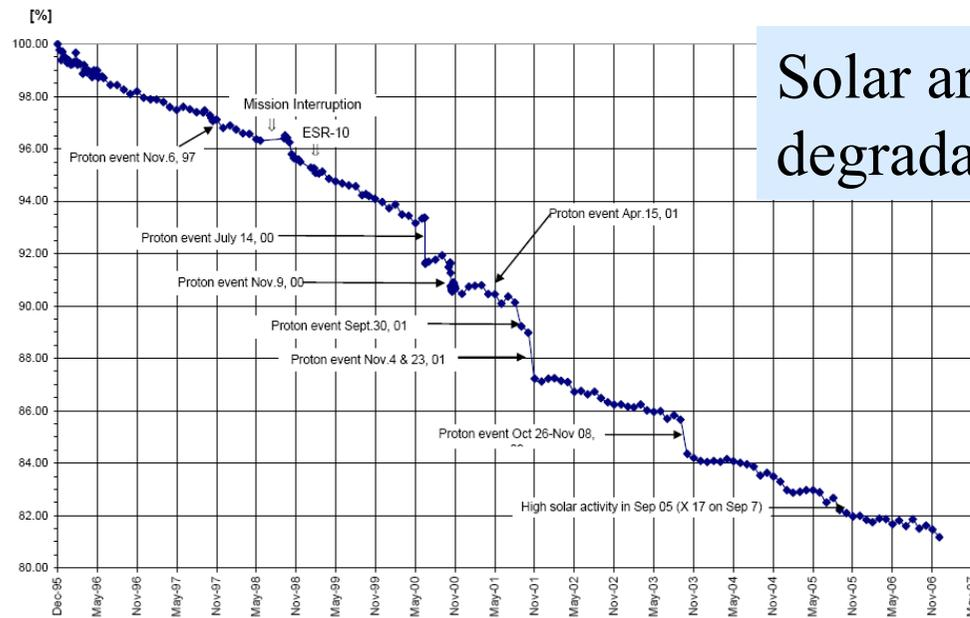
Solar array degradation
