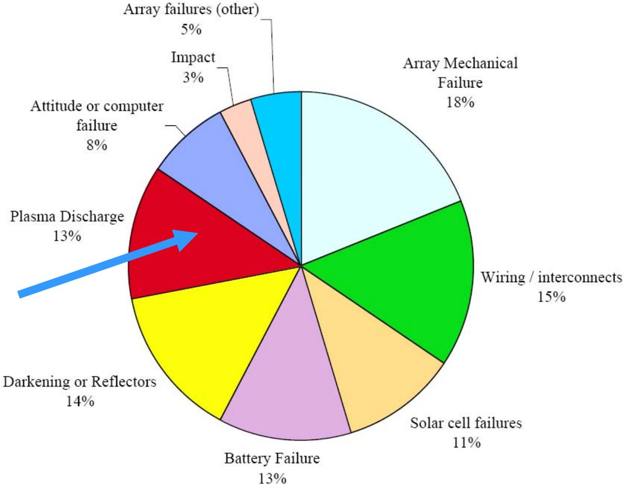
Figure 1. Number of power-related failures, by cause
