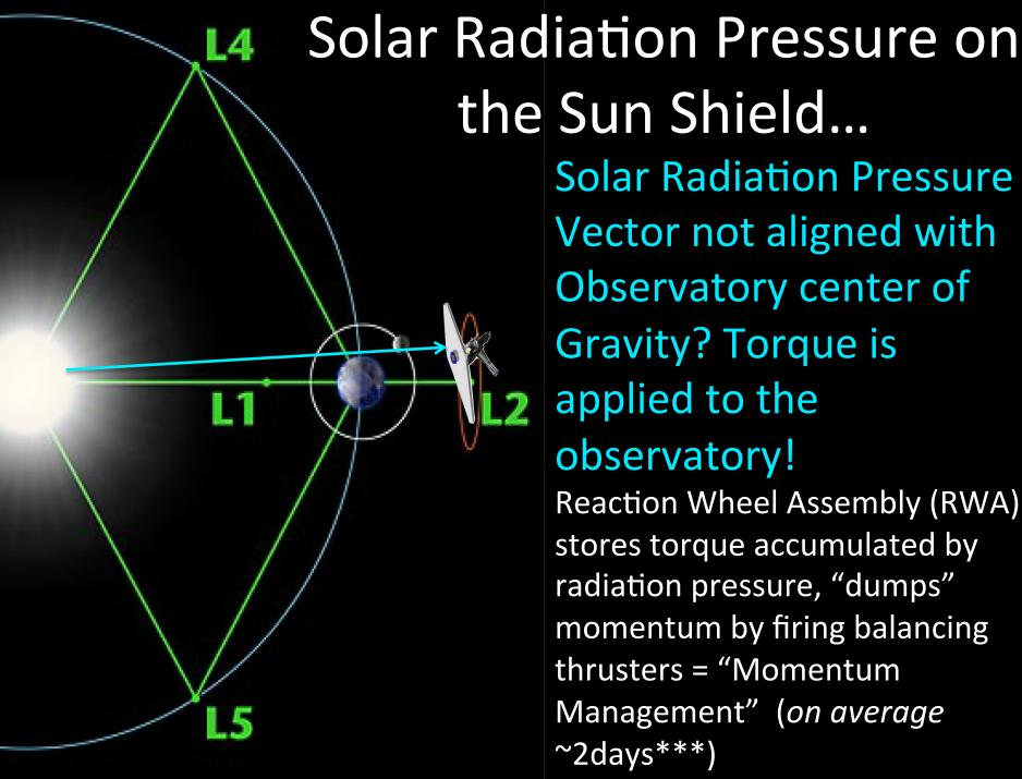
**Solar Radiation Pressure** Vector not aligned with Observatory center of **Gravity? Torque is** applied to the observatory!
