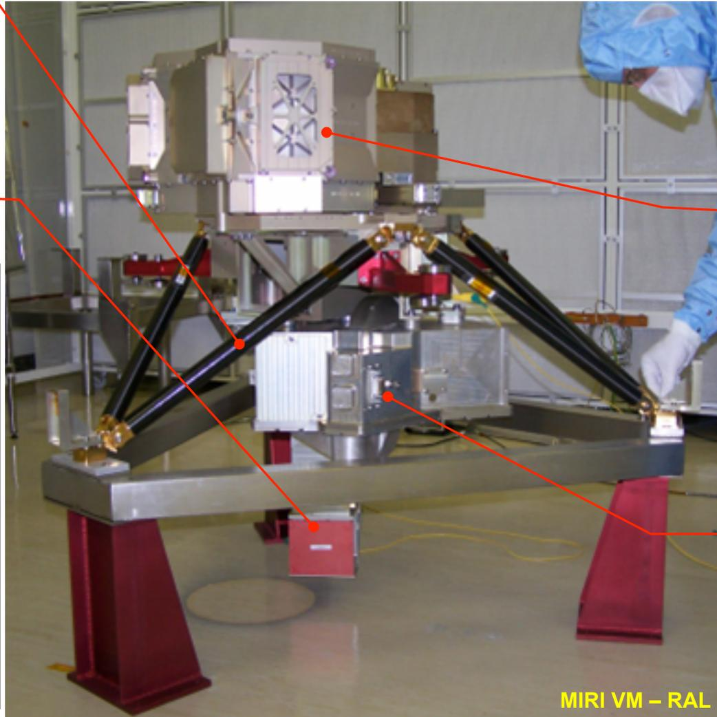
A 10 x 10 arcsec field passes through the deck into the R ~ 3000, 4 channel integral field spectrometer
