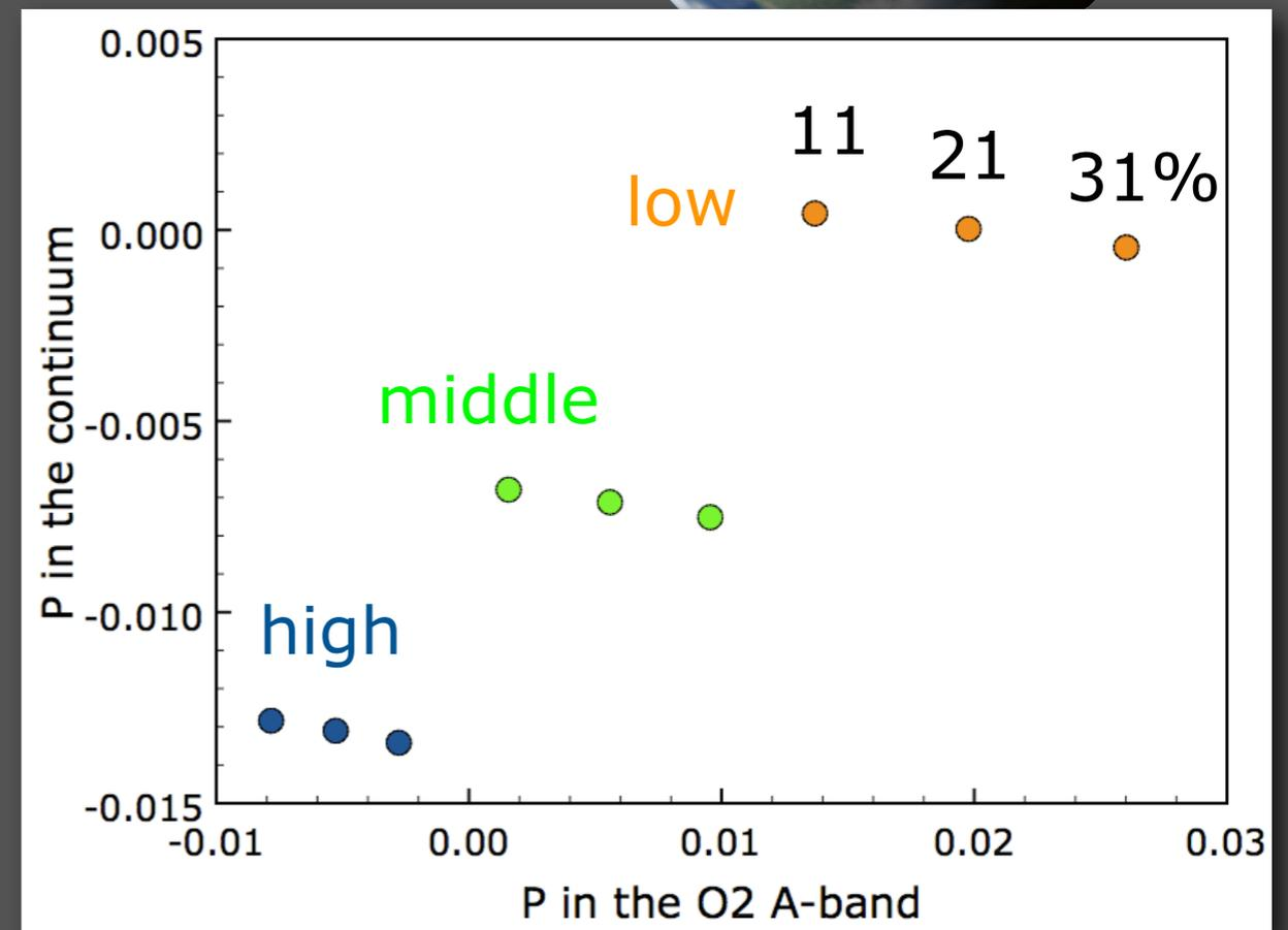
The reflected flux and degree of polarisation in and outside of the O<sub>2</sub> A-band (0.76 microns) for completely cloudy planets with high clouds (blue), middle clouds (green), or low clouds (orange) and for different O<sub>2</sub> mixing ratios (Stam et al., 2008)
