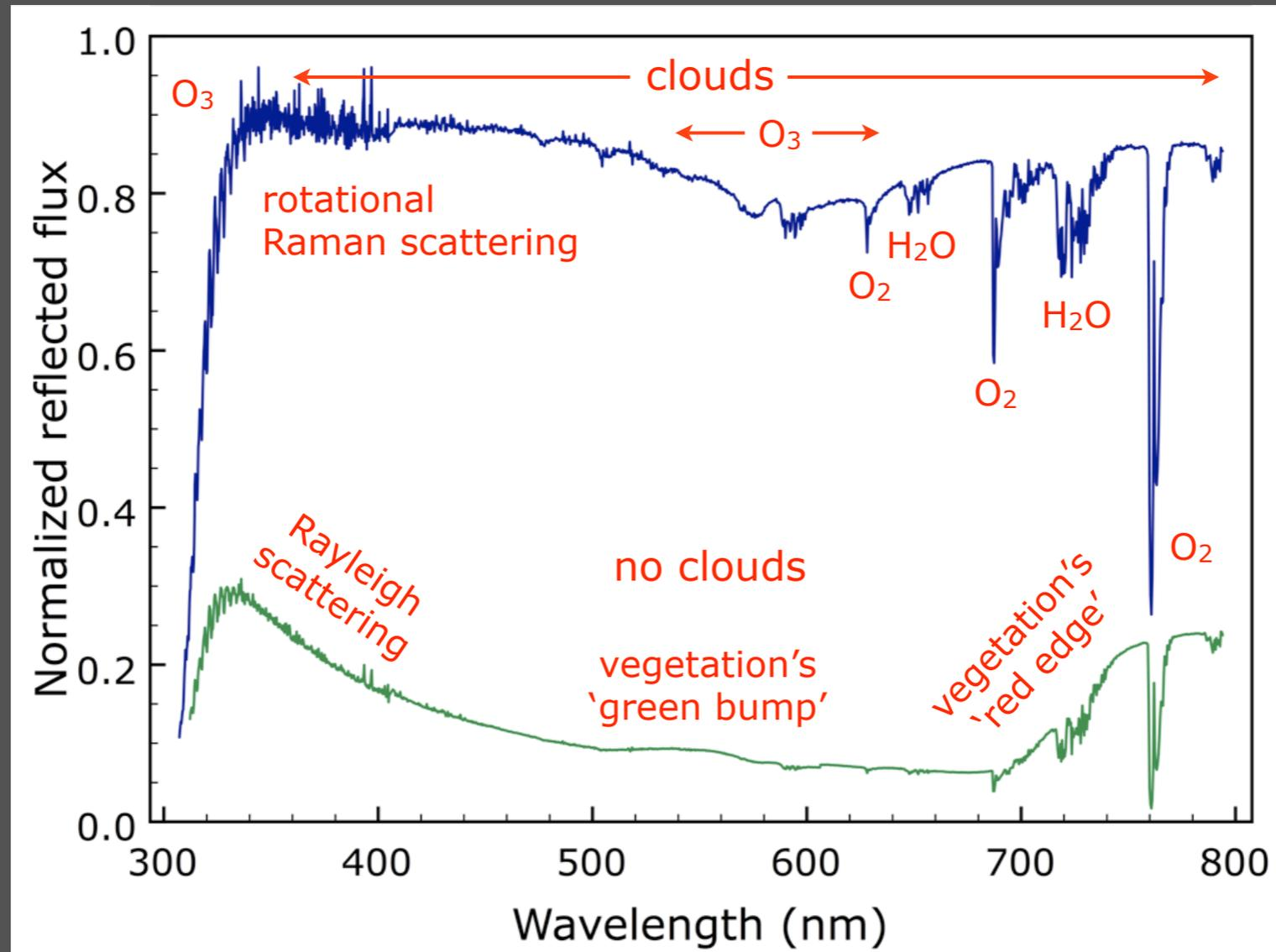
Spectrometry of a region on Earth measured by GOME on the ERS-2 satellite, for nadir viewing angles and solar zenith angles of  $34^\circ$
