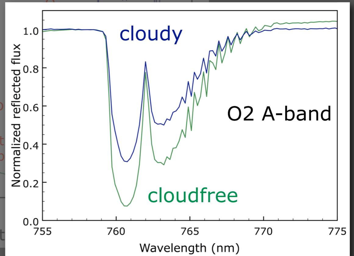
Spectrometry of a region on Earth measured by GOME on the ERS-2 satellite, for nadir viewing angles and solar zenith angles of 34°
