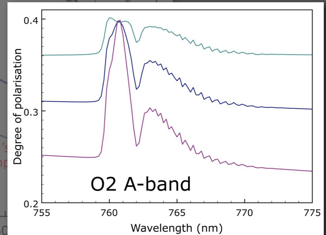
Ground-based polarimetry of the cloud-free zenith sky at three solar zenith angles  $\theta_0$  with the GOME BBM [from Aben et al., 1999]
