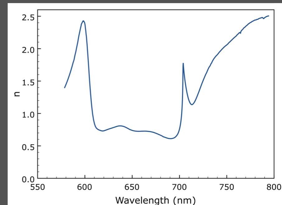
GOME's polarisation sensitivity (mainly due to dispersion gratings and dichroic mirror) (see Stam et al., 2000)
