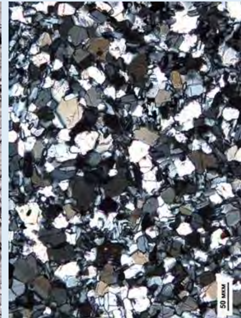
Luna 24 ferrobasalt thin section
