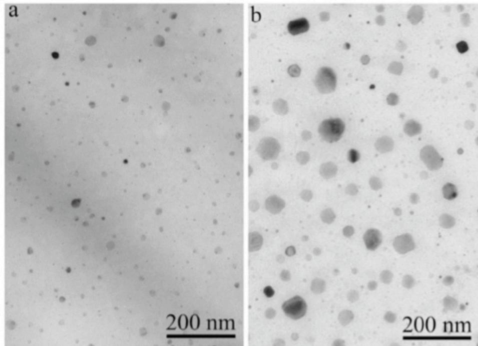
**Fig. 1.** TEM micrograph of annealed sample **a)** at 870 K for 780 h and **b)** at 1020 K for 3 h. Rounded metallic nano-particles enclosed in the amorphous silicate. They formed by a reduction reaction and further precipitation since metallic Fe is immiscible in silicates. The microstructure closely resembles to those to GEMS found in IDPs.
