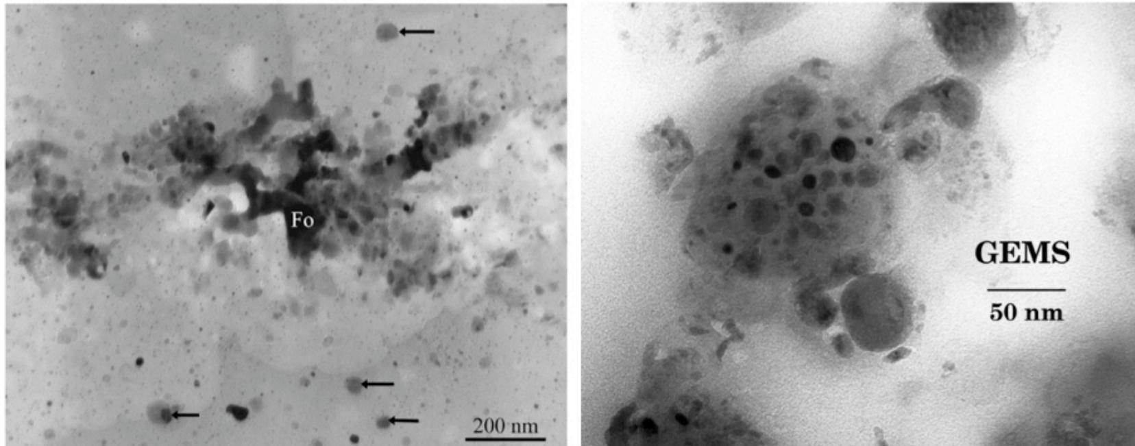
**Fig. 2.** TEM micrograph of sample annealed at 970 K (55 h) showing a forsterite crystal (Fo) embedded in a amorphous matrix. Note the dendritic structure at the edge of the grains. Some metal particles are also present in the amorphous phase (some of them are arrowed).
