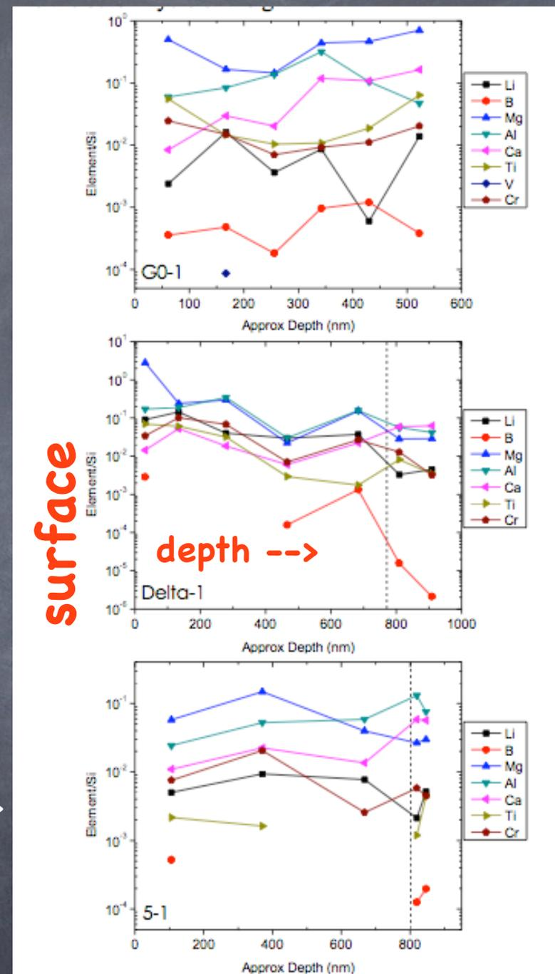
Figure 1. Examples of trace element depth-profiles which show either abundance peaks, are symmetrical, or vary little with depth. Dashed lines indicate the approximate depth at which the grain was removed from the TOF-SIMS and re-imaged.
