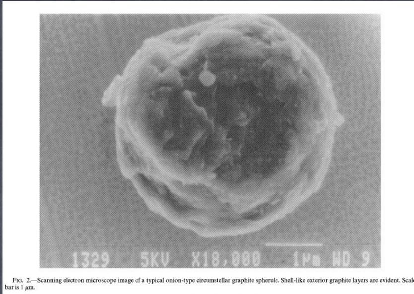
FIG. 2.—Scanning electron microscope image of a typical onion-type circumstellar graphite spherule. Shell-like exterior graphite layers are evident. Scale bar is 1 µm.
