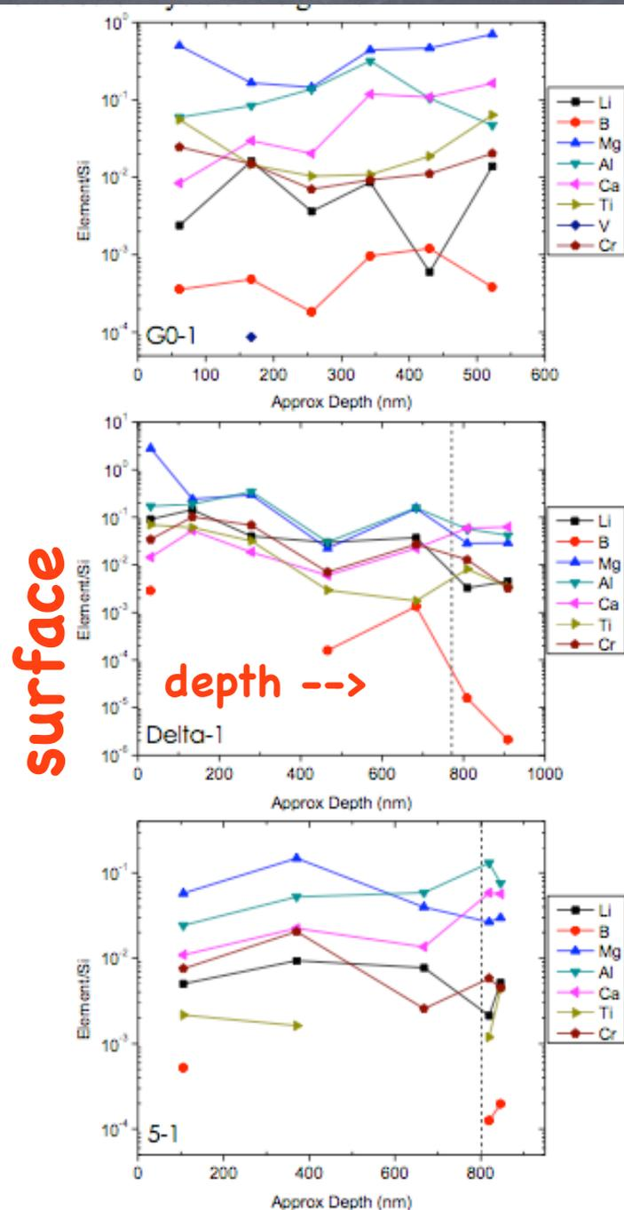
Figure 1. Examples of trace element depth-profiles which show either abundance peaks, are symmetrical, or vary little with depth. Dashed lines indicate the approximate depth at which the grain was removed from the TOF-SIMS and re-imaged.
