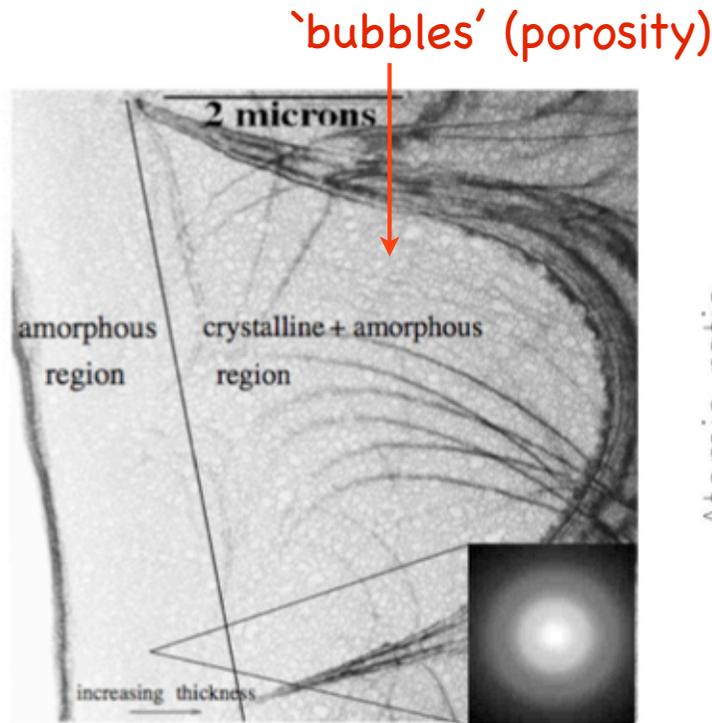
**Fig. 2.** TEM picture of a crystalline olivine sample irradiated with  $10^{18}$  10 keV  $\text{He}^+$ /cm<sup>2</sup>. The dark lines at the right hand side are Bragg diffraction lines. The picture in the bottom right is the electron diffraction pattern of the irradiated sample taken in the amorphous region. The observed diffuse halo is characteristic of an amorphous material. Note the presence of bubbles in the sample
