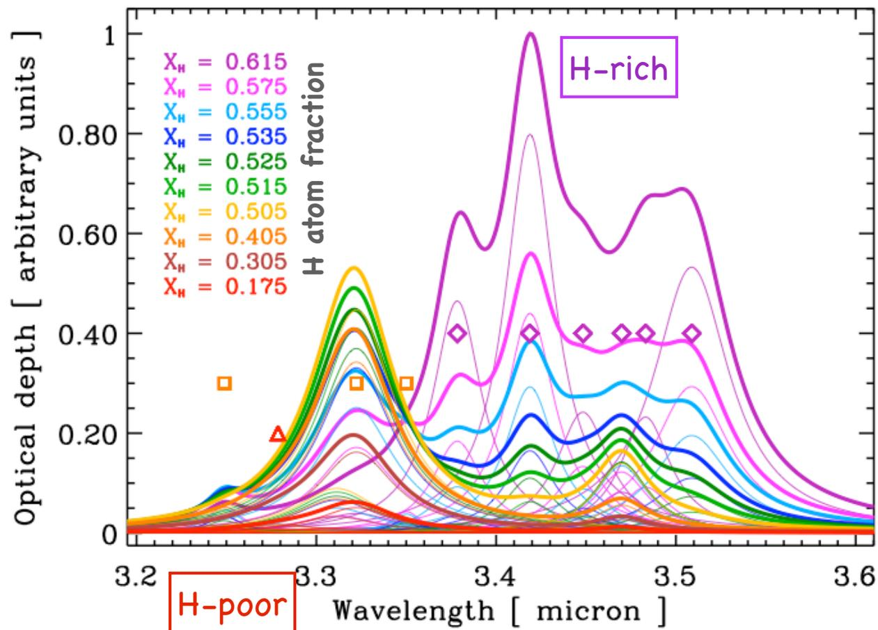
**Fig. 8.** The predicted eRCN spectrum in the 3.2 – 3.6  $\mu\text{m}$  C-H stretching region as a function of  $X_H$  calculated using the structural decomposition described in §2.2.3 and the data in Table 2. The diamonds, squares and triangles indicate the aliphatic, olefinic and aromatic band positions, respectively (see Table 2). Jones (2011a)
