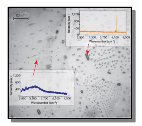
Synthetic fluid inclusions in olivine formed at 1,000 °C and 2.6 GPa at Fe–FeO buffer conditions. Three different types of fluid inclusions are visible. [...] These observations suggest that under run conditions, a hydrogenrich fluid phase coexisted with an immiscible water-rich fluid phase.
