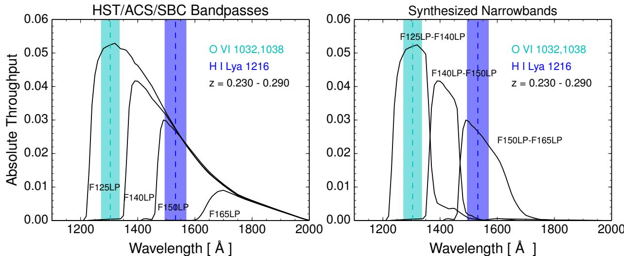
ACS/SBC LP filters: steep blue cut-on and extended red wing
