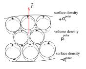
The atoms in a dielectric are modelled by electric dipole moments
